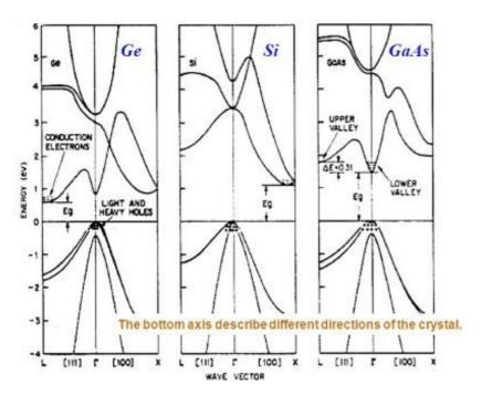
Shown above are the band diagrams for Ge, Si and GaAs. The number of valleys that exist at the conduction band minimum is
