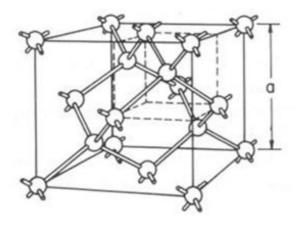
Given the side of silicon cube a = 5.43 A, what is the density of total number of electrons in the valence band of silicon in units of per cm<sup>3</sup>?
