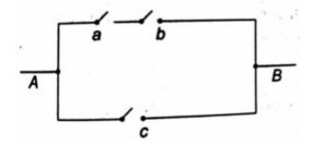
If the probability that each switch is closed is p, then the probability of current flowing through AB is
