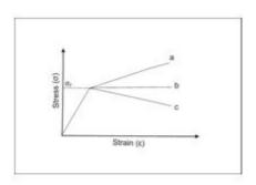
The above figure shows the flow behaviour of three plastic materials a, b, c. Which of the three substances show a 'strain hardening' nature?
