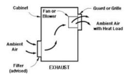
b) Each exhaust fan to be installed at 0.5 Feet below the level of the ceilings/roof. The Air Intake Fans should preferably be installed at a lower height from the ceiling and as much as possible be near to the
