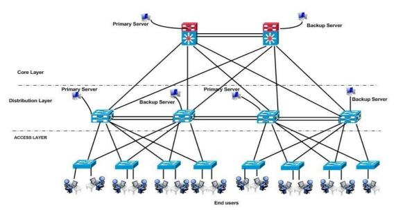
• Collapse core architecture in which both primary and secondary server connected to distribution switch in which no core switching place instead all access layer switches should connected to
