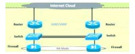
d) Scalability to provide Failover and Fall-back with alternate Service Provider, live or standby spare Router to be maintained as per business needs.
